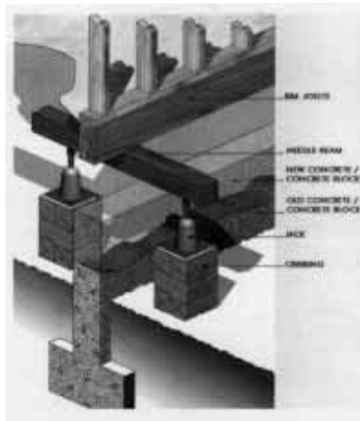
FIGURE 6. JACKING A WALL WITH PARALLEL JOISTS
