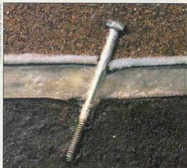
(Above) When hydrated, bentonite expands and conforms to penetrations and irregular surfaces, sealing small concrete cracks. (Right) Bentonite systems can be installed directly onto compacted soil or gravel substrate without a working mud slab.
